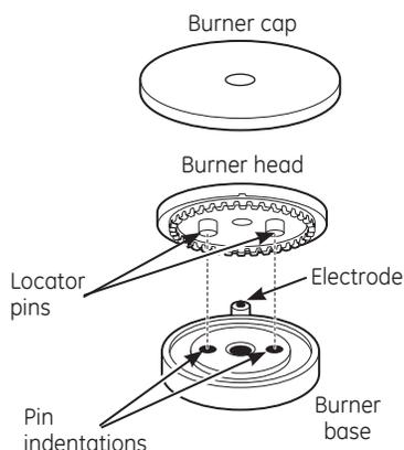
Make sure the pins in the burner heads match the burner base indentations and that they are properly seated in them by rotating the heads until they are level.
