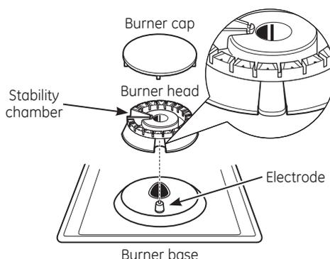
Make sure the slot in the burner head is positioned over the electrode. The burner cap has three to four pins. When replacing the cap, make sure none of the pins sits in the stability chamber.
