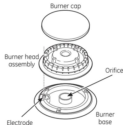
Make sure the hole in the burner head assembly is positioned over the electrode and that the burner head is fully inserted inside the burner base. A small gap between the base and head is normal.
