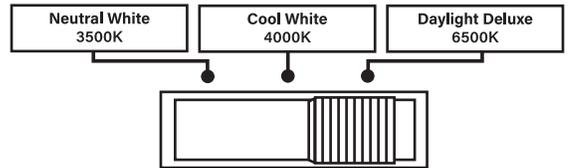
**NOTICE: The slide switch is located on the back of the lamp**
