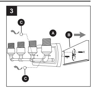
Feed supply wires through center of mounting plate (B). Attach mounting plate (B) to outlet box (not included) using the existing washers and outlet box screws or the machine screws (BB). Note: If the outlet box screws required for your outlet box are of a different size than the machine screws (BB), consult with a licensed electrician before proceeding.
