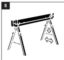
6. Legs adjust in increments of 1 inch. To extend, pull legs down until latch is locked at desired position. To retract, press lock button, pull legs down slightly then push leg up.
