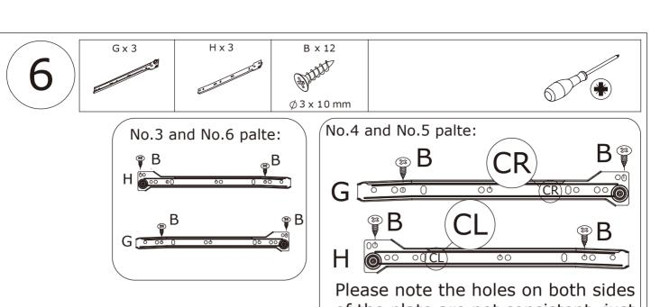
Please note the holes on both sides of the plate are not consistent, just for preventing the plate from being pierced by screws.
