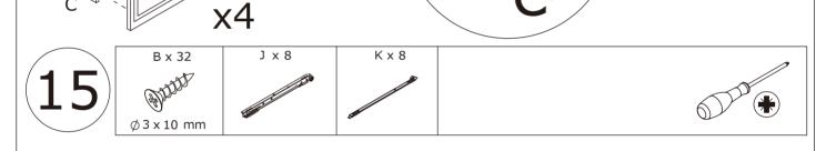
Fix runner(J) and (K) to No.15 and No.16 plate respectively with screw(B) as shown.
