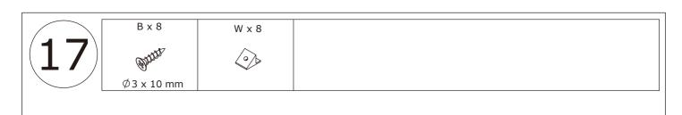
Insert buckle(W) into back slots and fix with screw(B) as shown.
