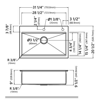
Model #: KWT300-32 Sink Dimensions: 31 1/4" x 20 1/2" x 9" Min Cabinet Size: 33"
