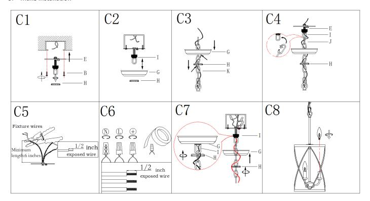
Step C1: Attach the single bar (E) to outlet box with mounting screws (B). The side of single bar marked "GND" must face out Unscrew the collar ring (H) from the collar loop
