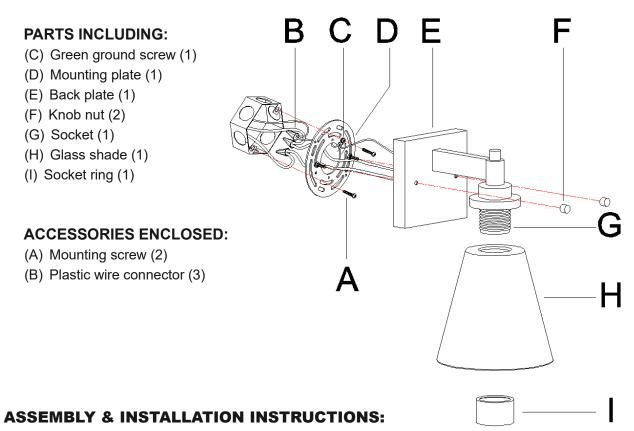
1. Carefully remove the fixture from the carton and check that all parts and accessories are included as shown in the above illustration.
