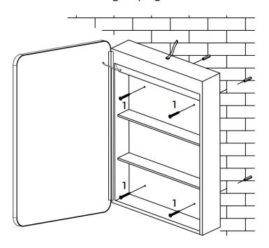
**Note:** When mounting to the wall, the wire can not be pressed between the cabinet and the wall, otherwise the wire installation will be affected.
