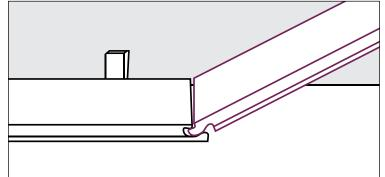
Start your second row. With a cut-off STEP that is more than 8" long or start with a new plank.
