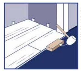
Step 1: Undercut space under door jamb to allow plank to slide freely. Tap long edge with hammer and tapping block to lock long edge.
