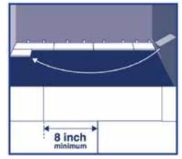
Step 3: Use leftover plank from first row as starter for second row. There must be at least 20cm between plank end joints on adjacent rows. FOR TILE INSTALLATIONS: The distance between end joints should be
