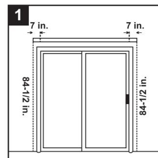
Next, place a light pencil mark on the front of the headrail (A) 7 in. in from each end. Hold the headrail (A) up to the sliding door at the height of the pencil marks on the wall. Center the headrail (A) over the top of the sliding door and use the pencil marks on the headrail (A) to make two more pencil marks on the wall.
