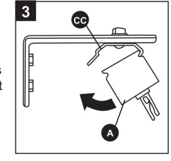
The headrail (A) is reversible depending on which side you would like to have the louvers (E) stack and where you want the wand (B) control. Center the headrail (A) under the mounting brackets (CC) and snap into position.
