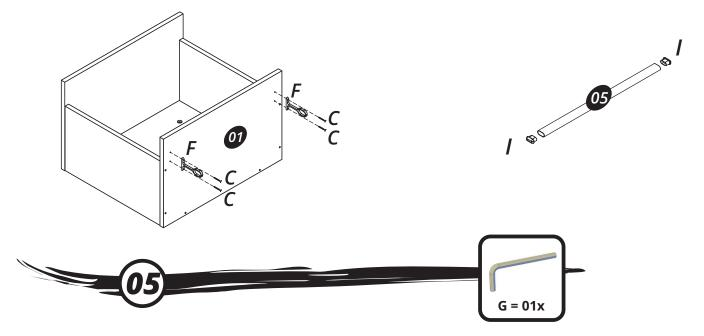
Pass the part (05) through the hardware (F) and use the hardware (G) to tight the screw as shown on detail.
