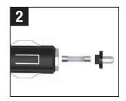
Remove and discard the old fuse. Insert the new fuse (either end).
