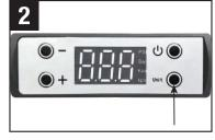
To choose and set the desired pressure format (PSI, BAR, KG/CM<sup>2</sup>, KPA), keep pressing the **Unit** button until the desired format displays.
