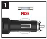
Carefully unscrew the front washer from the 12V DC Car Power Cord (it is spring loaded).
