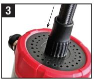
Connect the threaded metal end of the Schrader valve quick connector to the Inflator. Screw it in clockwise.
