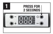
On the Control Panel, **press the & button for 2 seconds** to turn the inflator on. The LCD display will light up. Note: After 1 min of inactivity, the power will turn off automatically to conserve battery energy.
