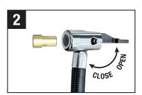
Flip the lever of the Air Hose Quick Connector into the up/open position. Slide the selected nozzle accessory into the Flexible Air Hose Quick Connector. Next, lower the lever into the down/closed position. This will create a seal and will hold the tip in place.
