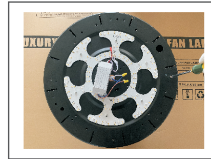
Step 4. Remove the main engine chassis screws.
