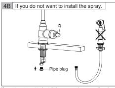
If you do not want to install the spray, please use the plug "L" to block-off and tighten it.
