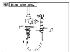
Insert spray seat through far right-hand hole on sink, then tighten mounting nut using adjustable wrench. Insert spray hose down through spray seat, then connect the spray hose to the outlet hose at the bottom of the tap and tighten it.
