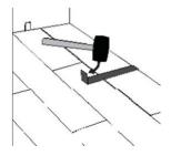
Step 9: Use hammer and pull bar to lock planks on final row
