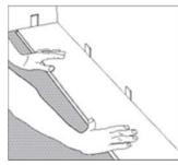
Step 1: Begin installation working from left to right. Insert spacers at ends and edges where planks meet wall to maintain ¼" expansion space
