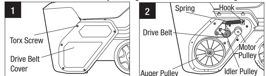
2. Remove the spring from the hook to release the belt tension (Fig. 3 & 4).
