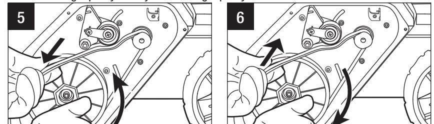
5. Use needle nose pliers (not included) to install the spring onto the hook to tension the drive belt (Fig. 3).
