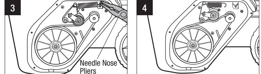
3. Remove the drive belt by slowly turning the auger pulley counterclockwise while pulling the belt outwards (Fig. 5).
