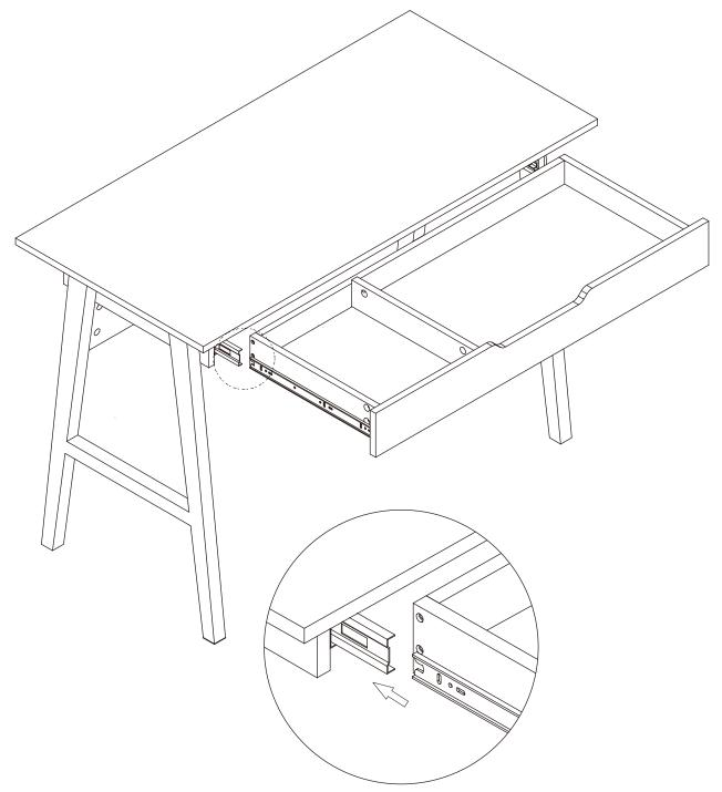
Note: Before installing the drawers, make sure the ball bearing piece is in the front end of the slide. After both sides are aligned with the guide rail, push the drawer along the guide rail.
