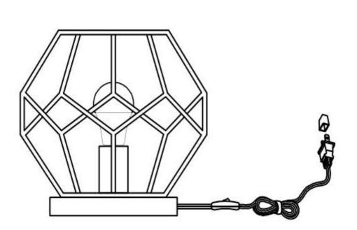
Step 1 Insert the bulb(D) into the socket(C).
