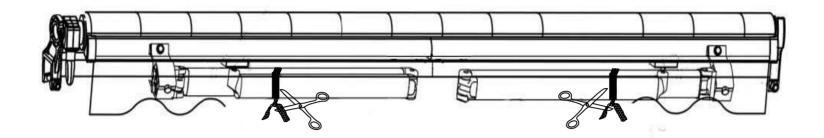
⚠ Cut off the bandings after the awning is fully assembled.
