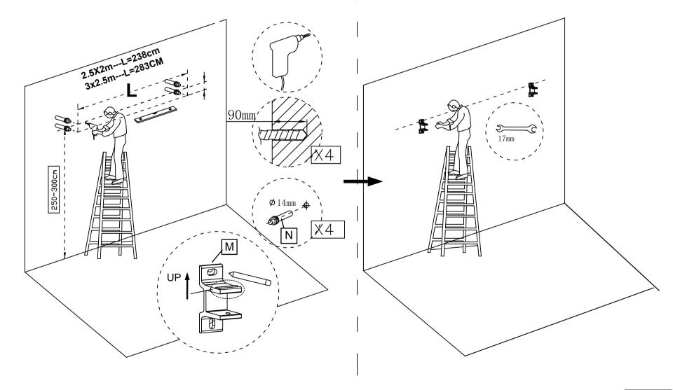
Install the awning on the wall bracket while tightening the fixing screws on the wall bracket. Locking plate
