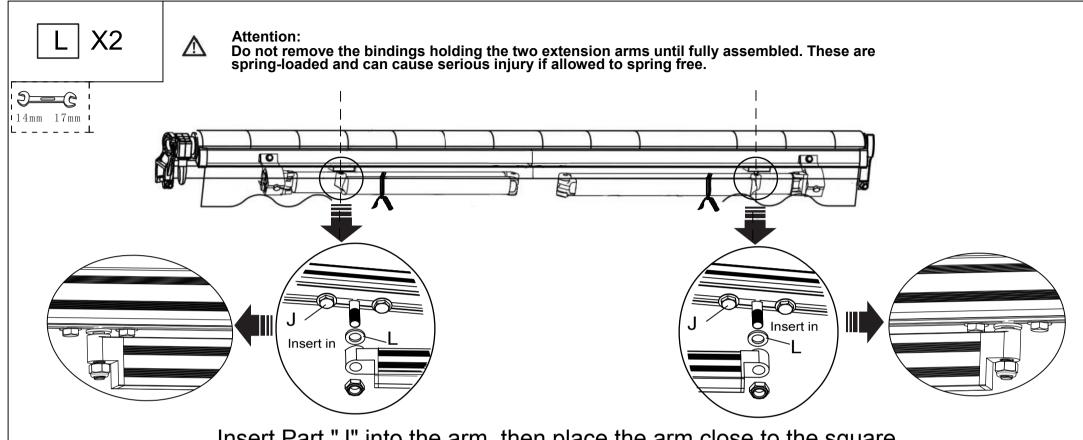
Insert Part "J" into the arm, then place the arm close to the square tube "B", keeping the arm parallel to tube "B" (this is an important step!!!)
