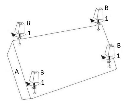
Place the Ottoman (A) on its back on a flat smooth surface. Attach Ottoman Feet (B) to Ottoman (A) and Washers (1) to each corner.
