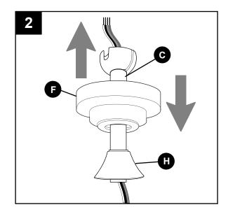
3. Slip downrod (C) into motor housing yoke, align holes and re-install pin (D) and clip (E). Tighten set screws in motor housing yoke and then tighten preassembled nut on one of the set screws. Then, slide yoke cover (H) and canopy (F) down until they rest on top of motor housing (I).
