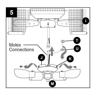
6. Locate BLUE and WHITE wires in switch housing on underside of motor housing assembly (I).
