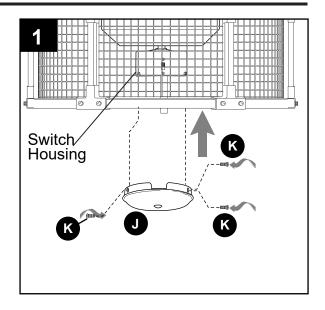
1. If you wish to use the remote control bracket from remote pack (G), install screws from remote pack (G) through bracket and into the desired installation site. The remote control transmitter from remote pack (G) rests inside the bracket.
