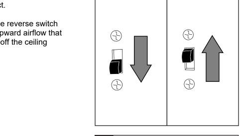
6c. **IMPORTANT:** Reverse switch must be set either *completely* UP or *completely* DOWN for fan to function. If the reverse switch is set in the middle position, fan will not operate.
