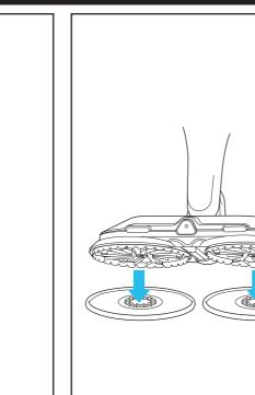
Insert the Mop Handle into the Steam Mop Body 2. To attach the Dirt Grip Soft Scrub Pads, place **BOTH** pads flat on the floor with plastic rings facing up. Align the unit directly over the plastic rings on the pads. Gently lower the Mop **Head** onto the pads, pressing until the pads are secure.
