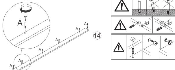
Screw eccentric rod(A) into board 14 at first. Attach board 14 to board 25, 2 and 26 using wooden dowel(H), add cam lock(B) into board 25,2,26 and turn clockwise to tighten as shown.
