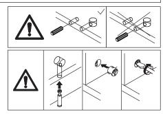
Connect board 6 to board 3 and 4 using wooden dowel(H), add cam lock(B) into board 6 and turn clockwise to tighten as shown.
