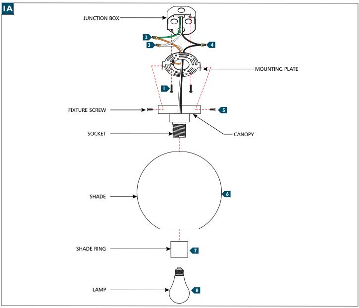
Secure the mounting plate to the junction box.
