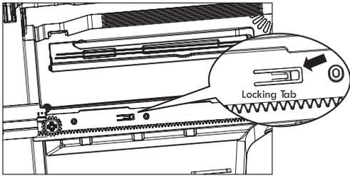
4. Pull exterior freezer drawer to fully disengage the rail assembly from the unit. Use 2 people for this task as the door is heavy and awkward to handle.
