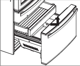
2. Remove lower freezer basket by pulling up and tilting toward refrigerator until it can be removed from the freezer drawer/door assembly.
