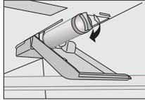
5. Dispense water over the course of 5 minutes in cycles of 30 seconds ON and 60 seconds OFF. Do not dispense water continuously for 5 minutes.
