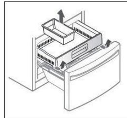
**CAUTION:** Pinch hazard! Keep hands and feet clear of the bottom of the freezer drawer when opening and closing.
