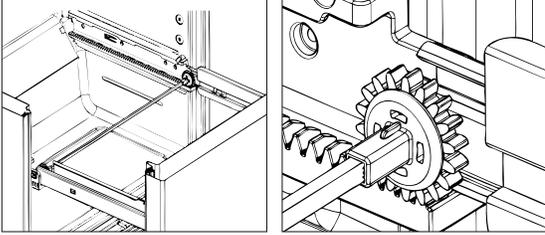
2. Fully push in and close freezer drawer to engage rails with rail support locking tab, applying a bit of pressure after the door is closed to seat the tabs to the rail.
