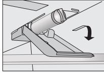
3. Remove the locking cap by turning 1/2 counterclockwise. Save locking cap for possible future use. Always install locking cap if no filter is in place.
