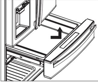
2. Pull back on the harness cover locking tab on left back side of pantry drawer front and remove the harness cover. Push down on tab on top of wire harness to disconnect it.
