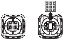
**NOTE:** Air Filter should be changed every 6 months. Replacing the water filter at same time as air filter is recommended.
