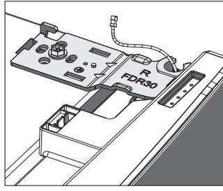
3. Screw top hinge cover into place with a screwdriver.
