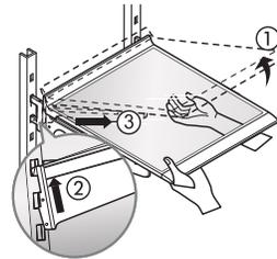
To reinstall a shelf: With front of shelf angled slightly up, engage hooks on back of shelf into attachment slots, and then lower front of shelf into place.
