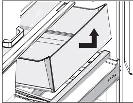
3. To install, slightly tilt up the front, insert the drawer into the frame and push it back into place.
