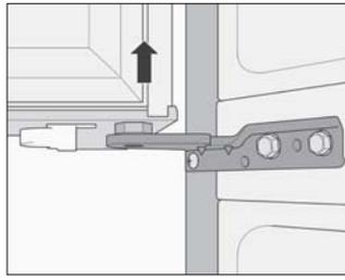
**NOTE:** If necessary to be able to move the unit through a narrow door or hallway, remove the left and right door middle hinges. Use a 10mm wrench to loosen and remove the two bolts attaching the hinge to the cabinet.
