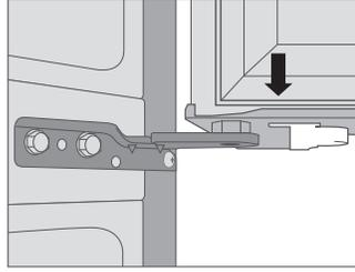
2. Fit the top hinge over the mounting holes and align to proper position before tightening. Use a 10 mm box end or socket wrench to turn top hinge clockwise to secure the hinge. Securely reconnect the wire harness.
