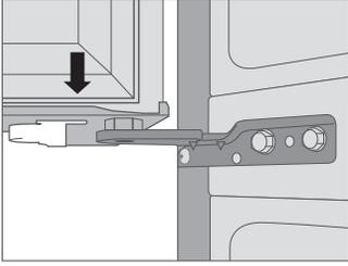
2. Fit the top hinge over the mounting holes and align to proper position before tightening. Use a 10 mm box end or socket wrench to turn top hinge fastener to secure the hinge.
