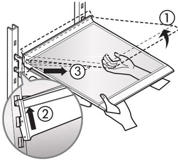
**To reinstall a shelf:** With front of shelf angled slightly up, engage hooks on back of shelf into attachment slots, and then lower front of shelf into place.
