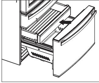
5. Open and close the freezer drawer several times to make sure operation is smooth and seal is consistent all the way around the freezer compartment.
