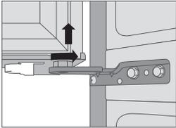
2. To lower a refrigerator door turn the screw clockwise.
