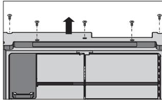
2. Using a 10 mm box end or socket wrench, turn top hinge fastener counterclockwise to remove the top hinge plate. Disconnect the wire harness.
