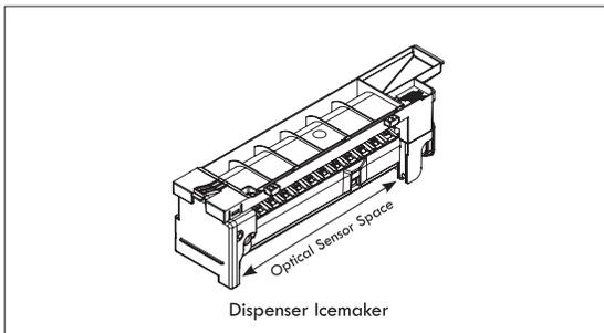
Icemaking will stop when the dispenser ice bin fills to the level of the optical sensor, or when the freezer ice bin fills and pushes the shutoff arm all the way up.
