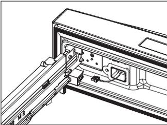
3. Use a 10 mm open end or socket wrench to remove the bolt connecting the rail to each side of the pantry drawer front. Tilt pantry drawer front up and remove from rails. Set pantry drawer front face up on a non-scratch surface.
