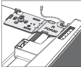
3. Lift the door from the middle hinge pin and remove the door. Place the door, inside facing up, on a non-scratch surface.
