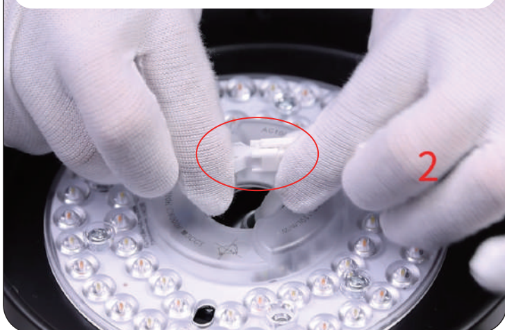
11. Connect the light source with the wires from the motor
