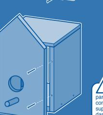
Attach the back shelves to the side panels using eight short nails as shown.
