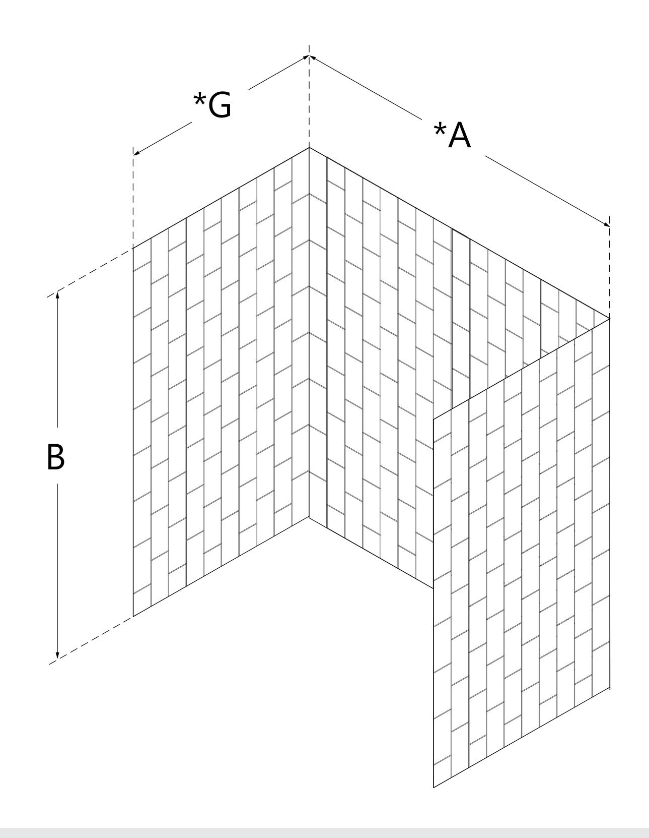
\*Panels trimmable from the edge that will be installed to the corner. Panel edges that will meet in the center of the wall should not be cut.
