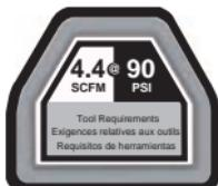
**IMPORTANT:** To operate correctly, this tool requires airflow that is at least 4.4 cubic feet per minute (SCFM) at 90 pounds per square inch (PSI). Check the specifications of your air compressor to be sure that it can support both the minimum SCFM and PSI required. The air hose length could affect how much air pressure the tool is actually receiving. You may need to adjust the air pressure higher on the air regulator to achieve the working pressure of 90 PSI.
