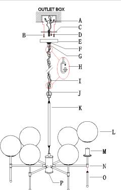
Step A1: Find out all the Tubes (O), secure all the tubes to the Lamp arms (N).
