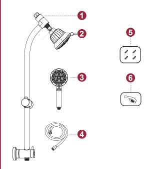
Apply teflon tape to shower arm. Attach the sliding bar with a built-in washer to the shower arm by rotating the hex nut clockwise by hand then lightly sung with a wrench.
