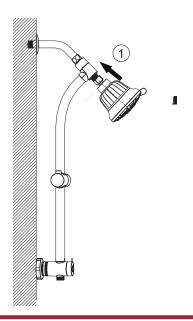
1. Attach the shower hose to the end of the sliding bar by rotating the hex nut of the shower hose by hand. 2. Connect the handheld shower and the shower hose by hand and put the hand shower into the slider.
