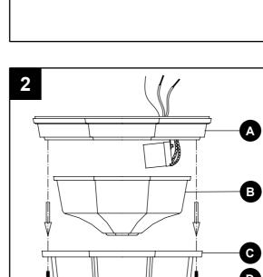
3. Strip 3/4 in. of insulation from wire ends. Twist stripped ends together with pliers (not included), black to black (power) and white to white (neutral). Attach copper wire to ground wire. **Helpful hint:** If necessary, attach copper ground wire to grounded outlet box.
