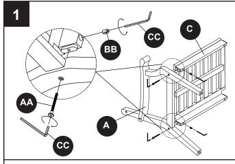
Once all bolts have been installed and hand tightened, go back and tighten firmly with wrench, CC.
