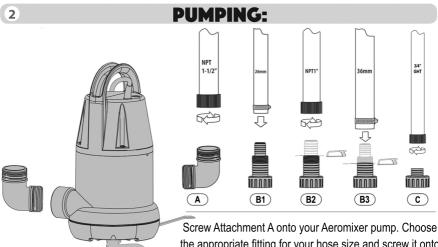
the appropriate fitting for your hose size and screw it onto Attachment A. If necessary, use a hacksaw or similar to modify Attachment B as pictured. Secure using hose clamp.
