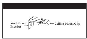
A. OUTSIDE MOUNT: Mount on a vertical surface (wall, window, or door frame) STEP 3A. The length of your blind is the exact distance from the top of your headrail to the bottom of the blade. Mark "HEIGHT" on wall at Vane Length plus (+) 2 inches.
