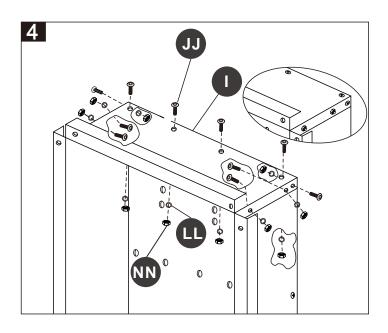
5. Attach the corner caps (B) to the front ends of cart bed using **four** sets of M6 x 12 mm screws (JJ), Ø6 mm lock washers (LL) and M6 lock nuts (NN). Then secure the rear ends of cart bed with another two sets of M6 x 12 mm screws (JJ), Ø6 mm lock washers (LL) and M6 lock nuts (NN). Tighten all hardware.
