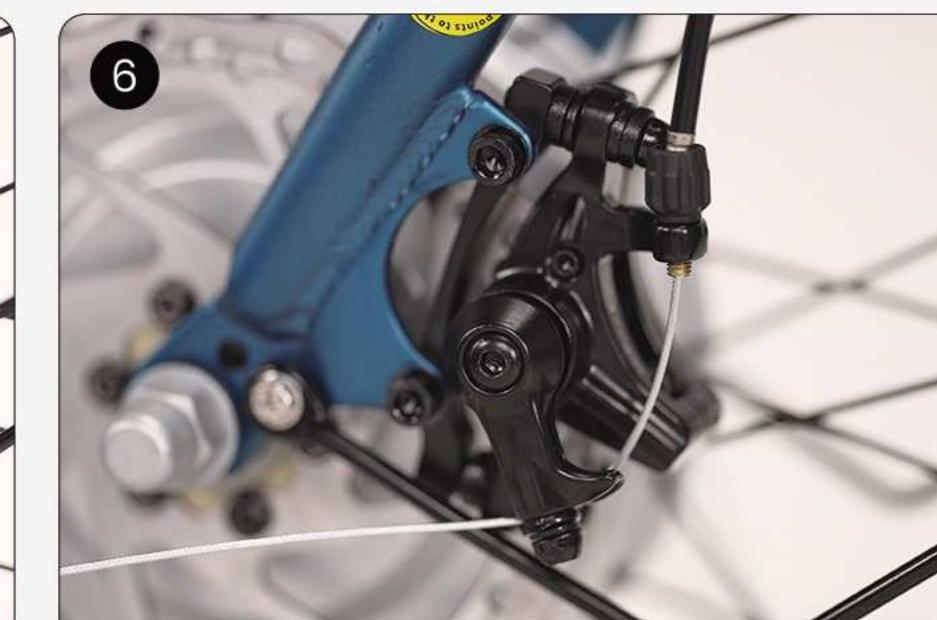
The front brake cable assembly is complete.
