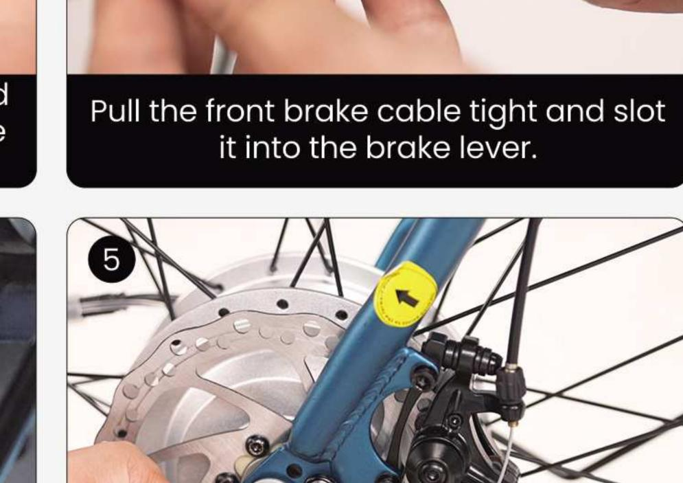
Thread the front brake cable through the Thread the front brake cable through the screw hole in the front disc brake and tighten slot in the washer screw and tighten the the screw to secure the brake cable core. screw to secure the brake cable.
