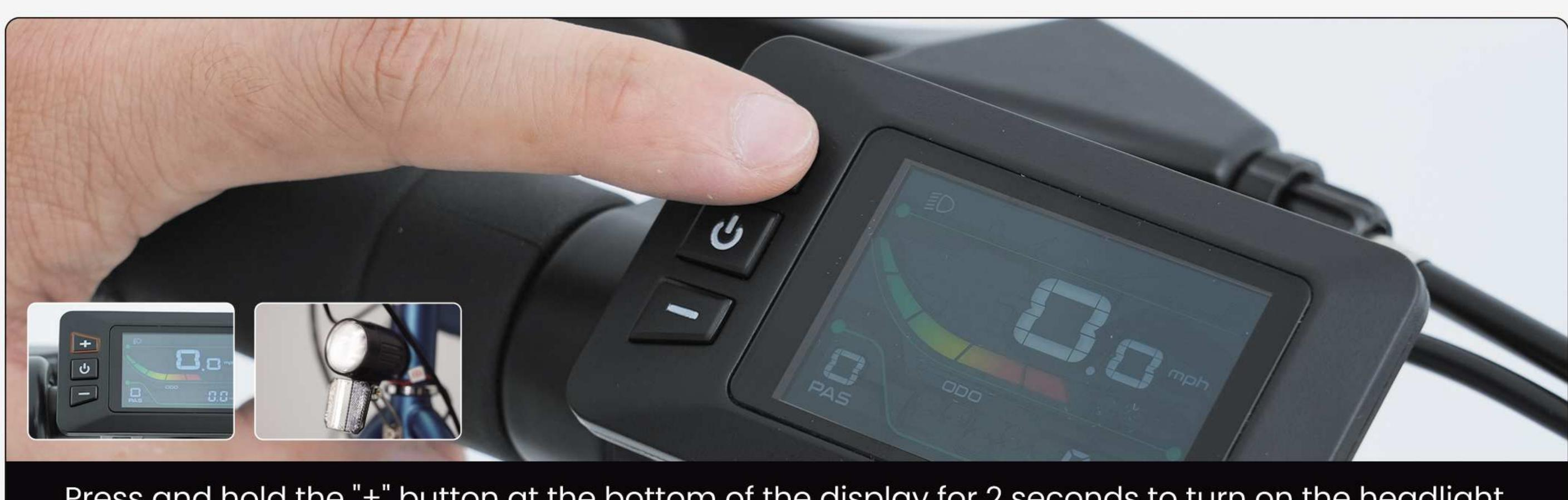
Press and hold the "+" button at the bottom of the display for 2 seconds to turn on the headlight. To turn it off, press the power button at the top of the display once.
