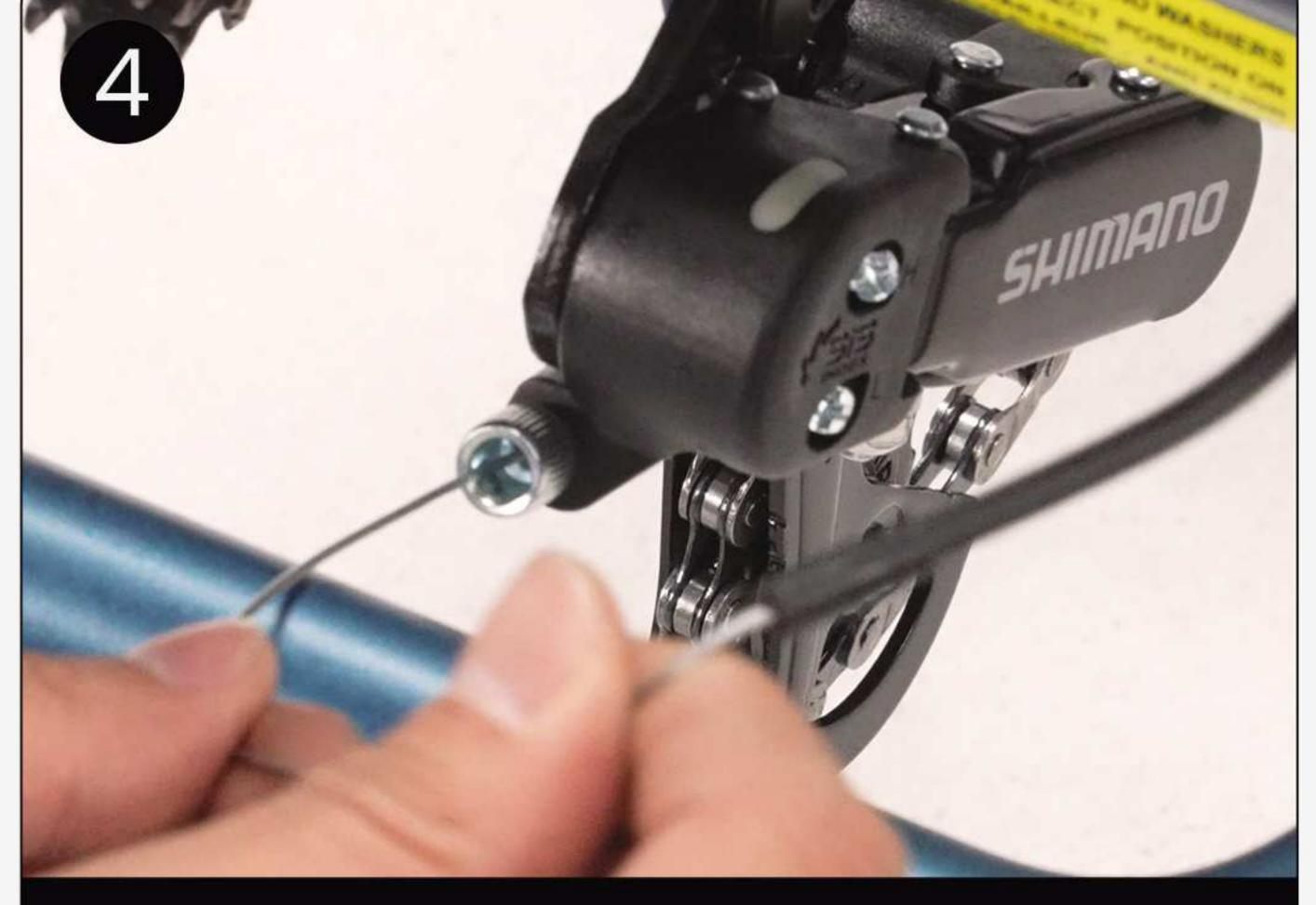
Thread the gear shift cable through the fine-tuning screw hole on the rear derailleur.
