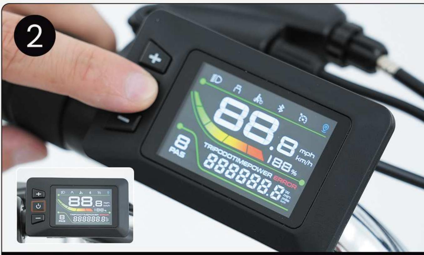
Press and hold the power button on top of the display for 3 seconds to turn on the screen; the display will light up, and the default gear will be "0," indicating the vehicle is in neutral.
