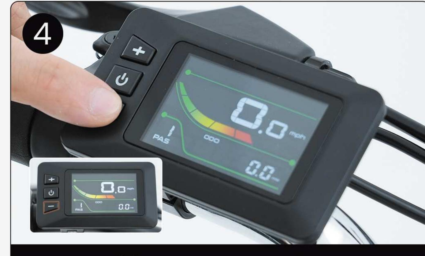
Press the "-" button below the display to decrease the gear, with a minimum of gear "0."
