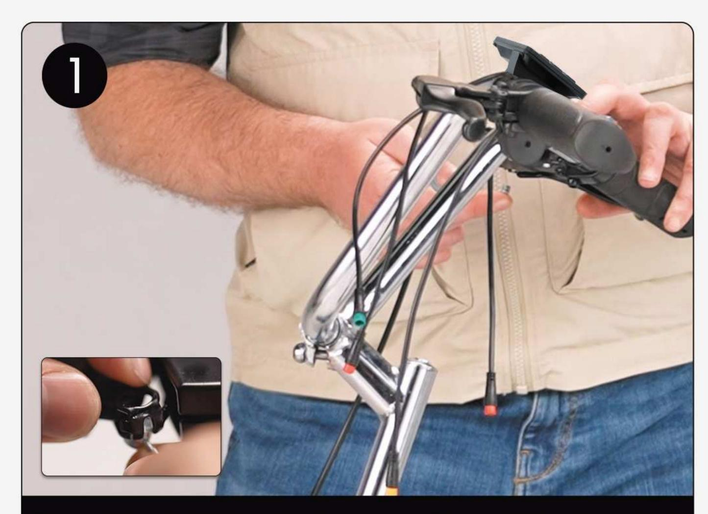
Press the right brake lever and insert the head of the rear brake cable into the lever hole.
