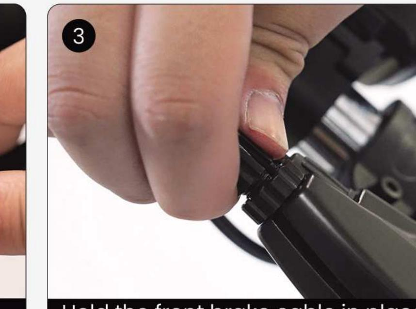
Hold the front brake cable in place and tighten the screw on the brake lever to secure the cable.
