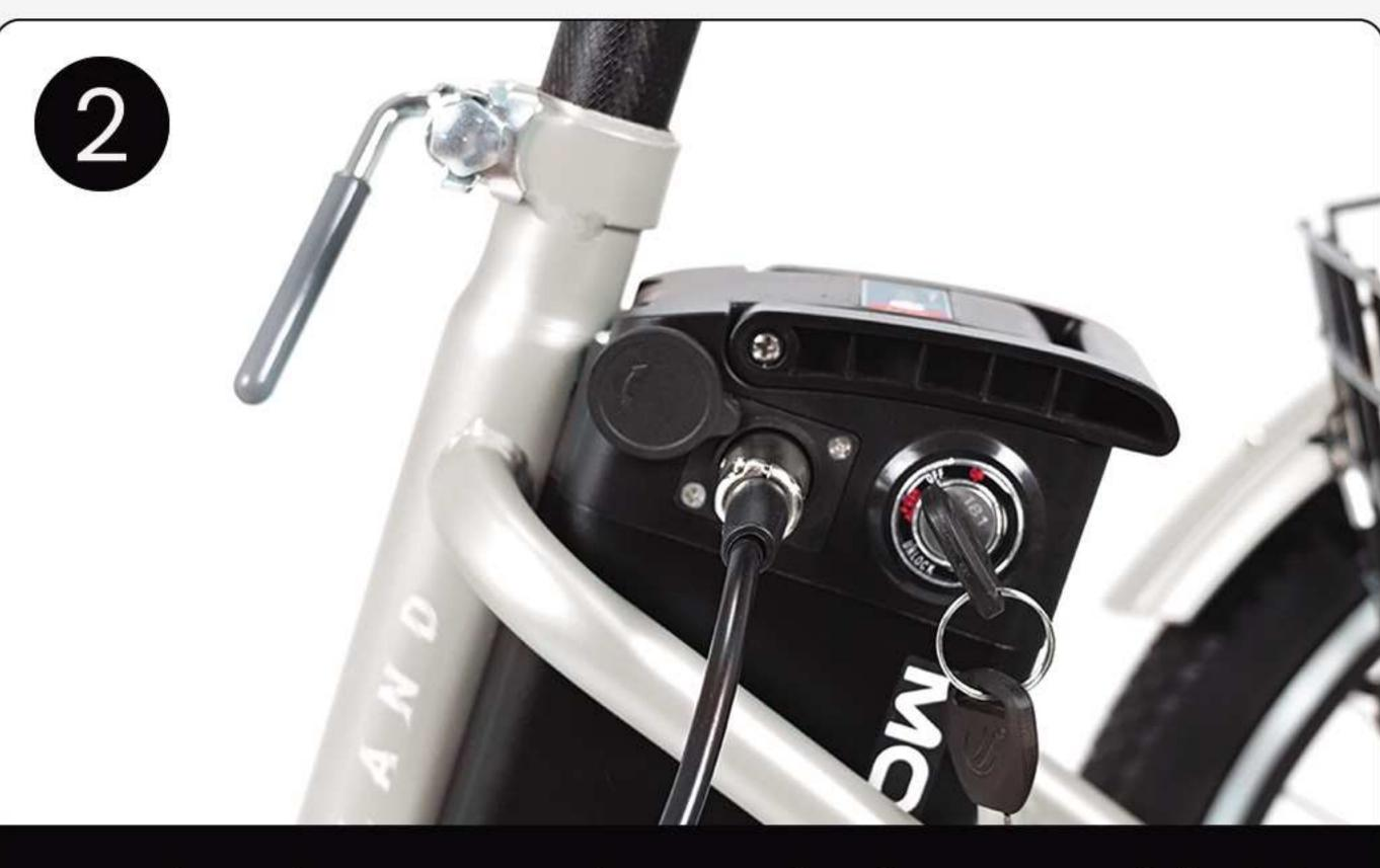
Use the charger to charge the battery while it is installed on the tricycle.
