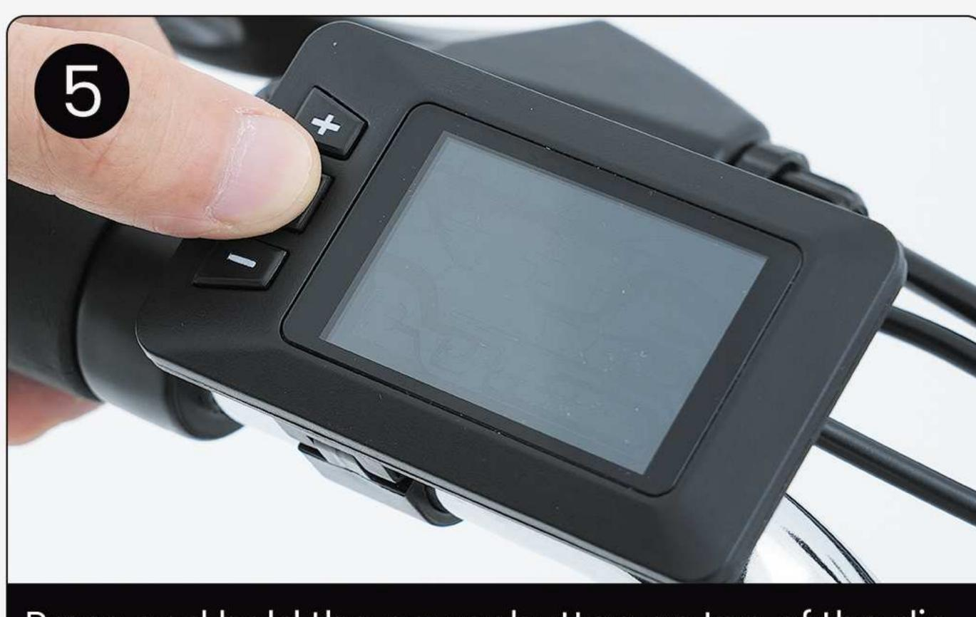
Press and hold the power button on top of the display for 3 seconds again to turn off the screen.
