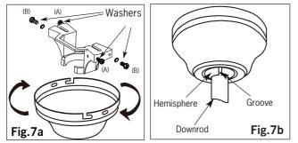
**NOTE:** When installing fan on sloped ceiling, make sure tab on hanger bracket faces towards the top of the slope. Depending on the slope, a longer downrod may be required to prevent fan blades from hitting the ceiling.
