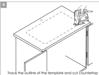
according to templated outline using appropriate cutting tools. Template is for guide only. Use physical sink to ensure accurate cut-out opening. It is recommended to use the actual sink dimensions to ensure the most accurate cut out. Drawing or template are for reference.
