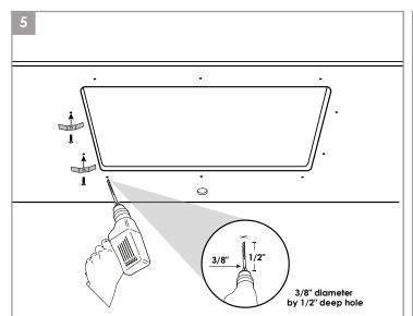
Drill holes on the underside of the countertop, approximately 1/2" from edge of the sink to be installed. Holes should be evenly spaced approximately 6" to 8" apart starting from every corner as shown below.
