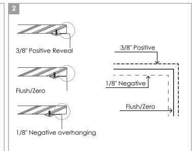
Use scissors to cut along the line of the paper template for you desired reveal type (Negative, Positive or Flush Reveal)
