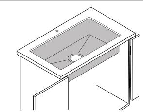
Check alignment of sink again and tighten fasteners to secure sink. Wipe away excess silicone caulk with damp cloth. Connect drain and water supply according to manufacturer's instruction.
