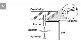
Option 1. Insert anchors under the countertop on the drilled holes, so they are ready to fasten the sink flange. Anchors should be inserted with a hammer until flush.
