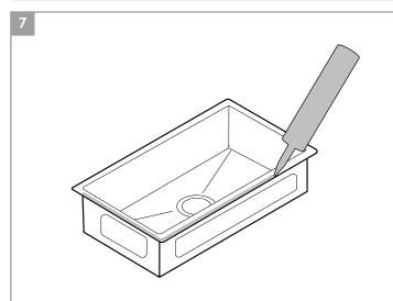
Clean sink flange and underside of cut-out area of countertop, making sure that the area is smooth and free of debris. Apply continuous bead of silicone caulk evenly on top of sink flange.
