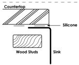
**Option 2.** Alternatively wood studs combined with silicone caulk can be used to hold sink against countertop without using mounting brackets.
