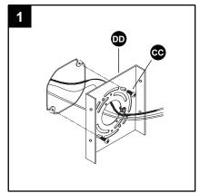
2. Strip 3/4 in. of insulation from wire ends. Twist stripped ends together with pliers (not included), black to black (power) and white to white (neutral). Attach copper wire to ground wire. Helpful hint: If necessary, attach copper ground wire to grounded outlet box.
