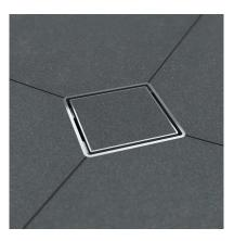
Step 2: Insert the stainless steel tray to be tiled into the stainless steel frame. Do not use any glue to attach tray to frame. The tiling of the tray may be done prior to this drain cover assembly. After cleaning the tray from grease, oil or other contaminants, you may adhere tile using wedi joint sealant or 100% Silicone (spot bonding without sealing over water relieve holes in tray) or modified, cement based tile adhesive (full surface skim coat of a compressed thickness of 1/8" max.).
