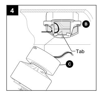
4. Temporarily hang fan on the tab on the mounting bracket (B) using one of the non-slotted holes in the canopy (C).
