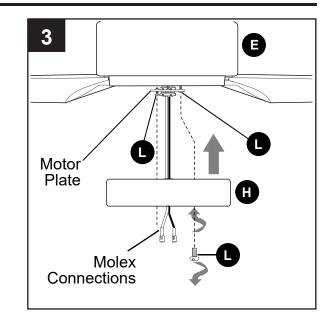
Partially loosen two fitter plate screws (M) in metal posts on underside of the fitter plate (H) and remove the other fitter plate screw (M).
