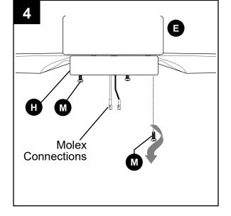
Connect WHITE wire from LED light kit (G) to WHITE wire from motor housing (E). Connect BLACK wire from LED light kit (G) to BLUE (or BLACK) wire from motor housing (E). Make sure molex connections snap together securely.
