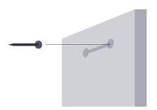
Then simply use the slot to move and center the plaque.
