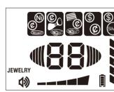
01 Press PP button, "PP" on LCD flashes. When LCD displays steady "PP", you can start to move the search coil slowly above the sound area. If the detector finds the target, it sounds a tone. Also the digital value of the target and depth are displayed on LCD.
