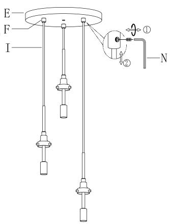
5 » If needed, shorten the extra length of the fixture wires from cord (I) so that they all are at least 6 inches (152.4 mm) long above canopy (E) within the outlet box.
