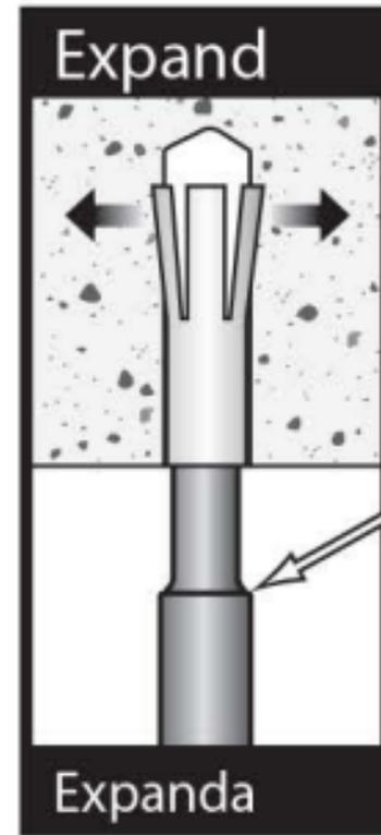
Expand anchor with the Red Head Setting Tool until shoulder of tool is flush with the end of the anchor.
