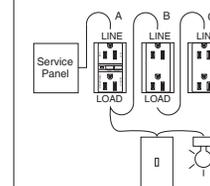
Always place Outlet Branch Circuit Type AF/GF in position A. All outlets of the protected branch, including lighting and receptacle outlets, must be connected to the load side of the AF/GF.
