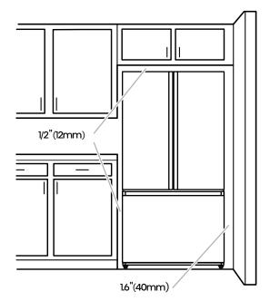
To ensure proper ventilation for your refrigerator, allow for a 1/2"(12mm) space on each side and at the top.
