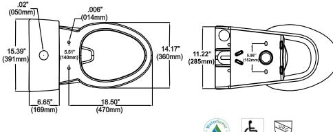
NOTE: All dimensions are in inches and millimeters. Illustrations may not be drawn to scale. IMPORTANT: Dimensions of fixtures are nominal and may vary within the range of tolerances established by ANSI Standard A112.19.2 These measurements are subject to change or cancellation. No responsibility is assumed for use superseded or voided.
